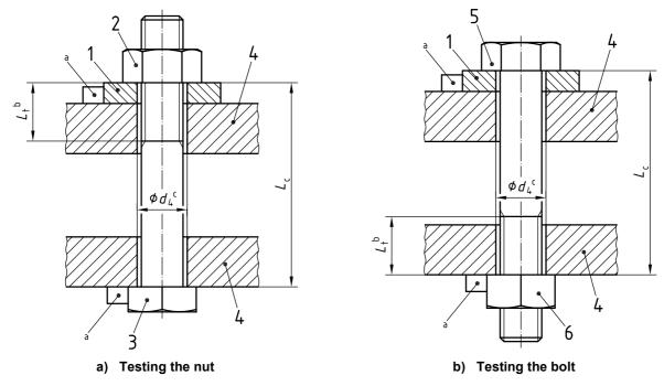
For testing studs, a fixture and setup of test specimen similar to a) is used. However, only the nut end should be tested. Before testing, the metal end of the stud shall be prevented from rotating.
