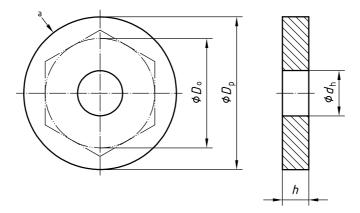
The outer contour of the test-bearing plate or test washer is not specified. It shall, however, have a plain surface with a diameter  $D_{\rm p}$  larger than the outer diameter  $D_{\rm p}$  of the bearings surface of the bolt, nut or washer of the screw and washer assembly to be tested.
